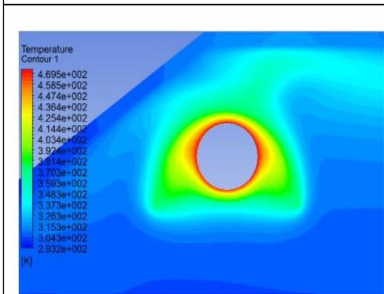
Fig. 6: Temperature contours in the cavity receiver (without radiation heat loss, absorber tube temperature 200°C)
