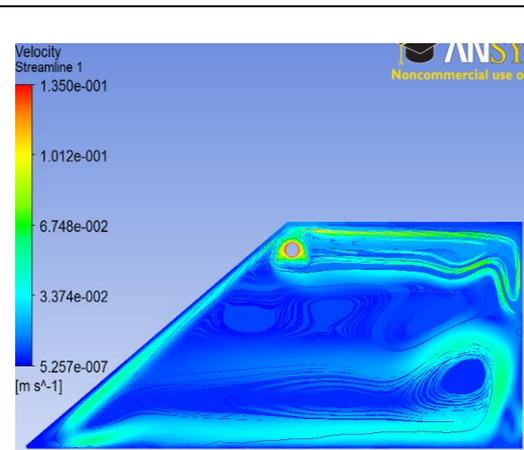
Fig. 5: Velocity streamlines in the cavity receiver (with radiation heat loss, absorber tube temperature 200°C)
