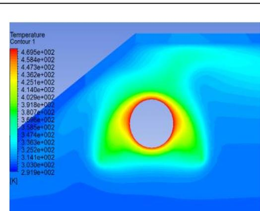
Fig. 7: Temperature contours in the cavity receiver (with radiation heat loss, absorber tube temperature 200°C)
