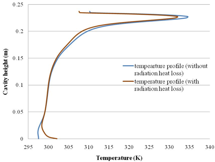
Fig. 12: Temperature profile within the cavity for absorber tube temperature of  $200^\circ\text{C}$  (with and without radiation heat loss)
