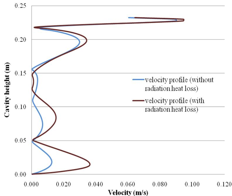
Fig. 13: Velocity profile within the cavity for absorber tube temperature of 200°C (with and without radiation heat loss)
