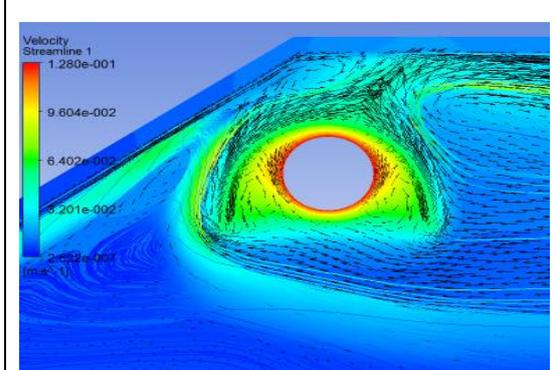
Fig. 8: Velocity magnitude contours and vectors in the cavity receiver (without radiation heat loss, absorber tube temperature 200°C)
