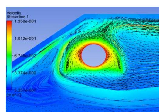
Fig. 9: Velocity magnitude contours and vectors in the cavity receiver (with radiation heat loss, absorber tube temperature 200°C)
