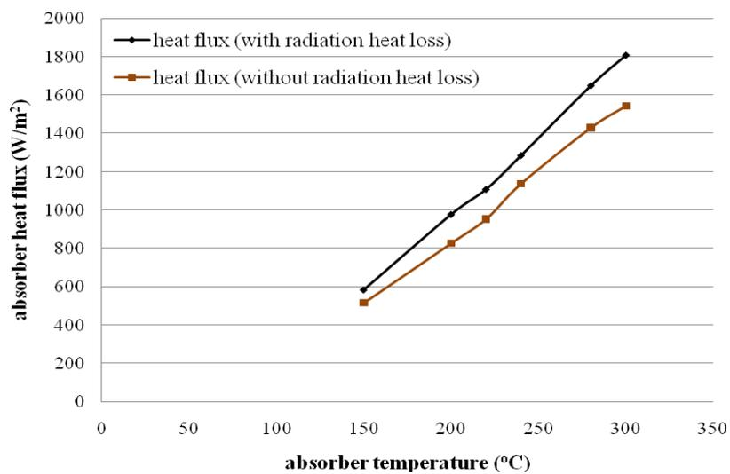
Fig. 10: Absorber heat flux (W/m<sup>2</sup>) showing the effect of radiation heat loss
