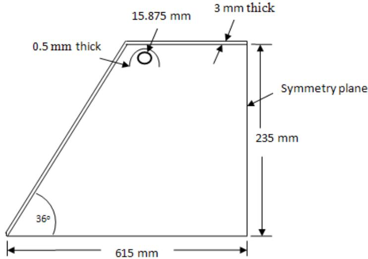
Fig. 3: Cavity geometry
