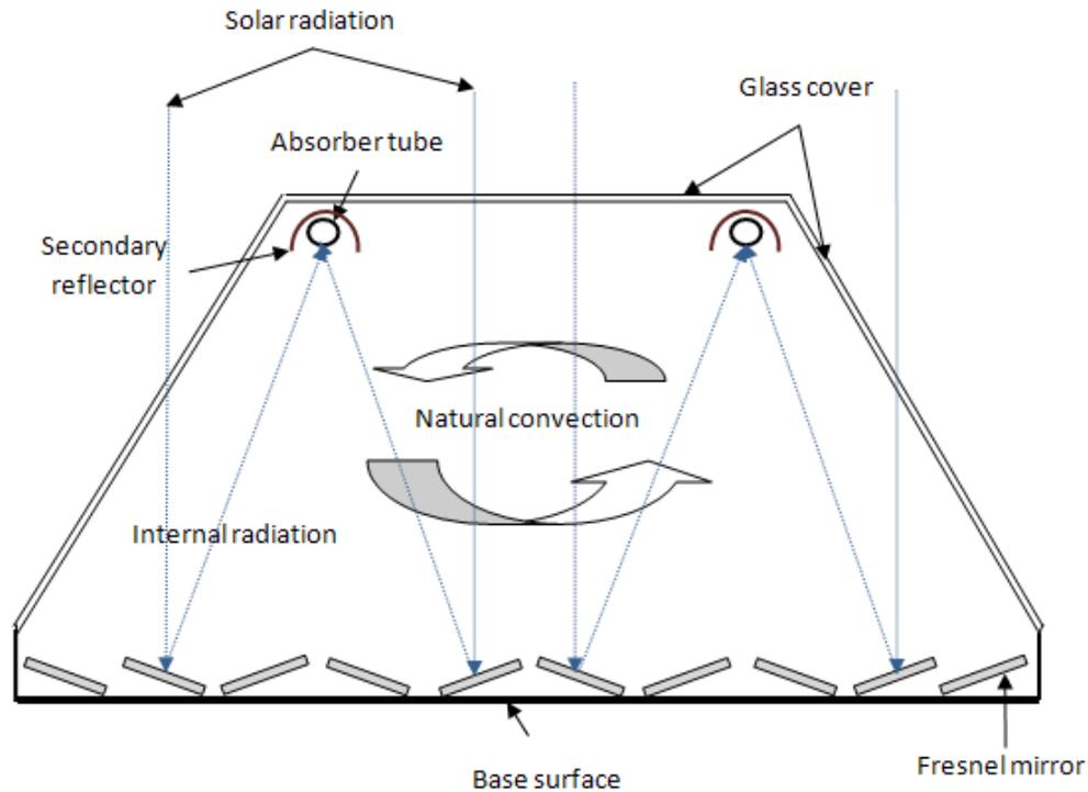
Fig. 2: Cross-section of the receiver cavity of micro-concentrating collector
