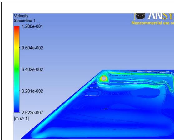
Fig. 4: Velocity streamlines in the cavity receiver (without radiation heat loss, absorber tube temperature 200°C)
