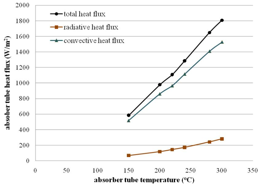
Fig. 11: Absorber heat flux per unit of absorber area ( $\text{W/m}^2$ ) for different absorber temperatures
