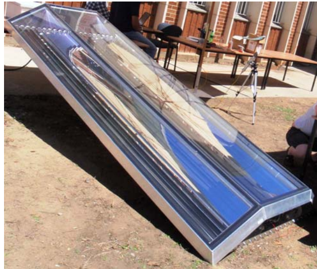
Fig 7: The prototype hybrid CPV-T MCT system on-sun and tracking.
