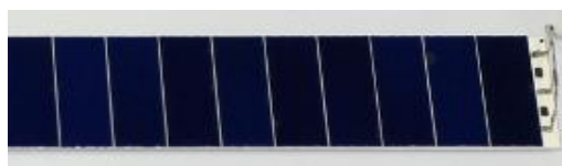
Figure 5: Close-up of an un-encapsulated section of an MCT sub-module.
