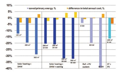
Among the large-scale systems, the PV-supported system offers a higher percentage of primary energy savings (blue to purple bars) at a lower cost (yellow-orange bars) than a solar thermal system of comparable size. This trend is reversed in the smaller systems.
